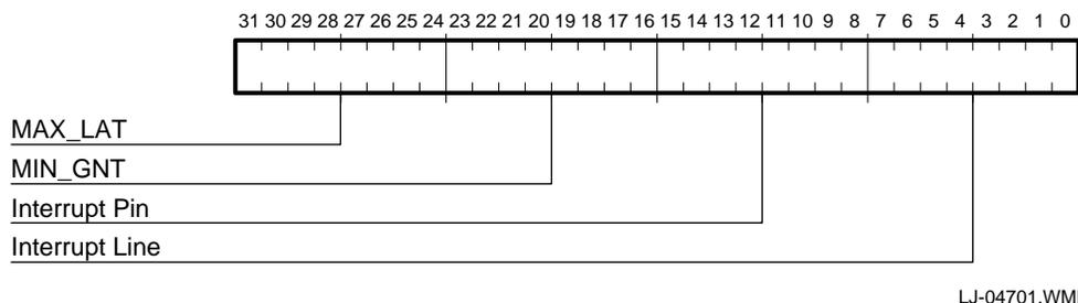
**Figure 3-13. CFIT Register Bit Fields**
