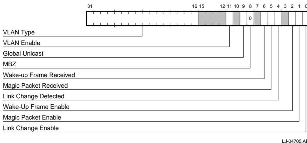
Figure 3-31. CSR2-PM Register Bit Field
