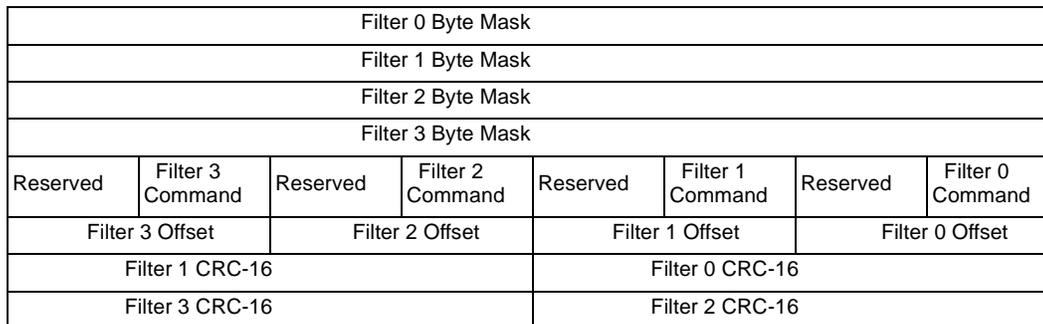
Figure 3-25. Wake-Up Frame Filter Register Structure
