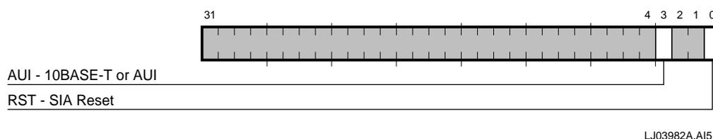
**Figure 3-42. CSR13 Register Bit Fields**
