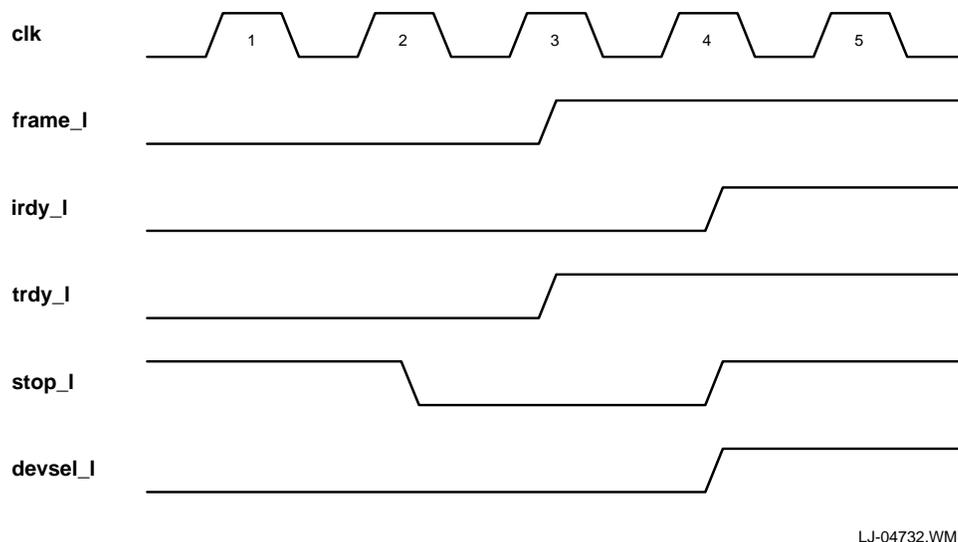
**Figure 5-12. Target Disconnect**
